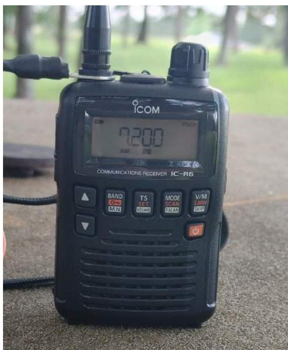
**Using a small receiver that can tune HF may help you discover noise ahead of time if you scout a location. Pay attention to antenna polarization, vertical antennas often find noise.**
