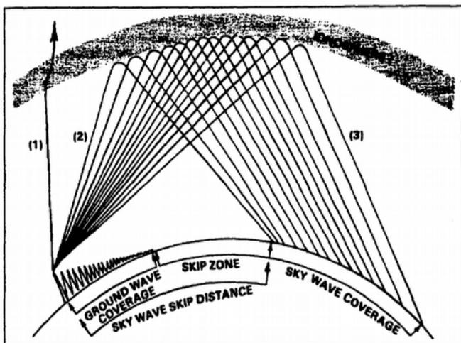
Figure 3-6. Relationship between skip zone, skip distance, and ground wave.
