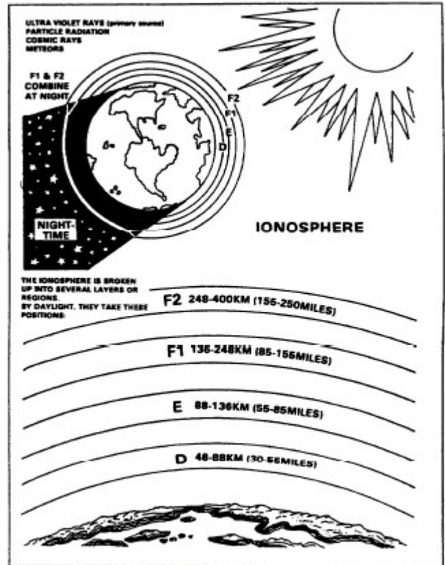
Figure 3-1. Layers of the ionosphere.
