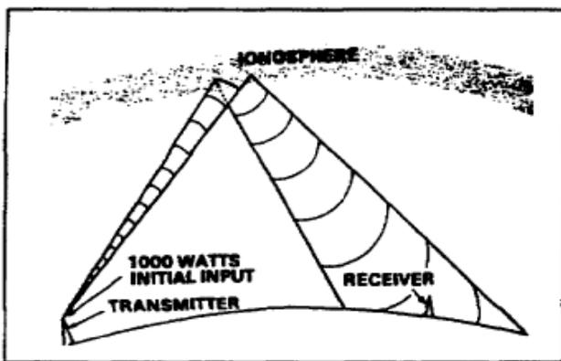
**Figure 3-8. Free space loss principle.**
