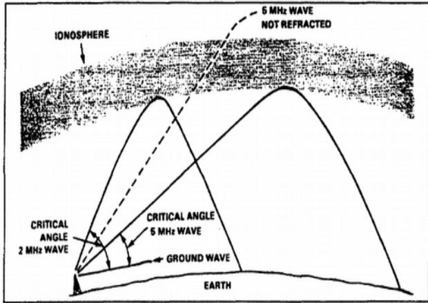
Figure 3-5. Effect of frequency on the critical angle.
