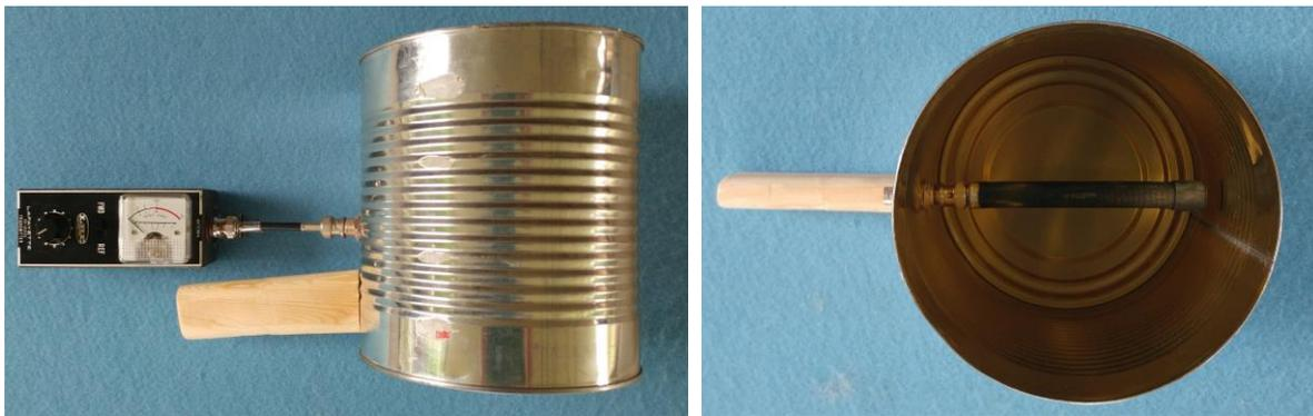
This is a single 1 gallon tomato can and the probe is a short  $\lambda/4$  ducky. The meter is an old SWR meter that has a BNC Field Strength Antenna input.
