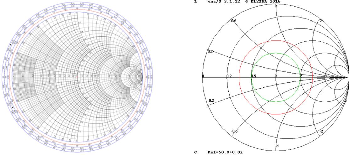
The **Smith chart** was invented 1939 by Phillip H. Smith. This graphical chart was originally designed to assist radio frequency (RF) engineers in solving problems with transmission lines and matching circuits. The Smith Chart shown above on the left side reminds me of the Slide Rule I used 60 years ago before invention of the electronic calculator. Today, most instruments that display Smith Charts, the graph will look like the one shown on the right side.
