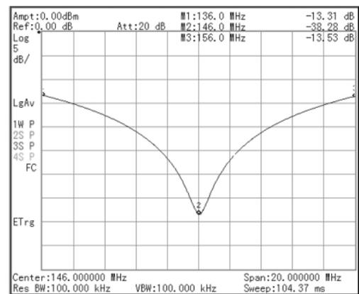
The resonant frequency of this  $\lambda/4$  wavelength cable shown on page 1 was 146.0 MHz, but the insertion loss was 13.5 dB because of the cables Q value. The term "Q" is a dimensionless value defining a "quality of merit" of tuned circuits. For a cavity, Q is a measurement of its narrow bandwidth of either pass or notch capabilities. The Q value of cavities depends on the cavity body diameter which range from 4 to 10 inches.
