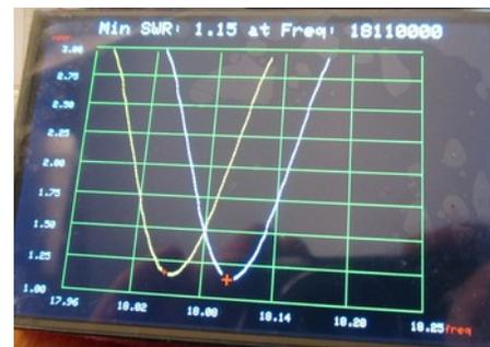
Figure 9. Overlay scan plot.
